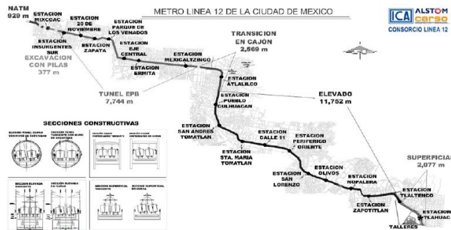
Figure 1. Line 12 layout with its construction zones (Benamar y Zaldívar, 2010).
