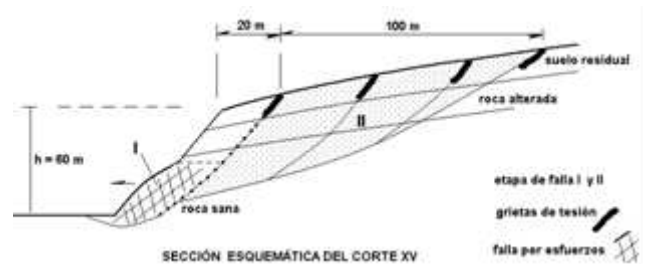
Figure 8. Schematics of the failures occurred in Cut XV
