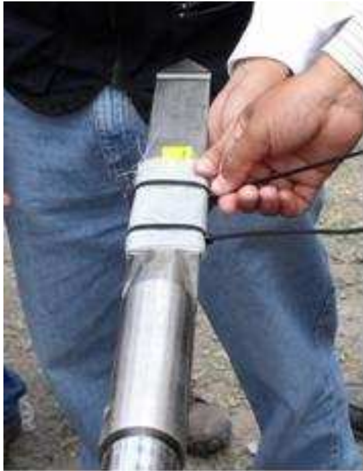
Figure 2. Protecting the piezometer of the piezo-cell
