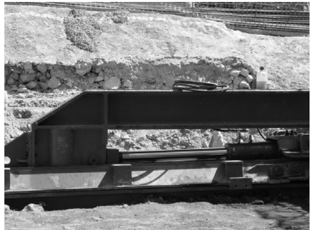
Figure 12. Detail of one of the thrust cylinders SS500
