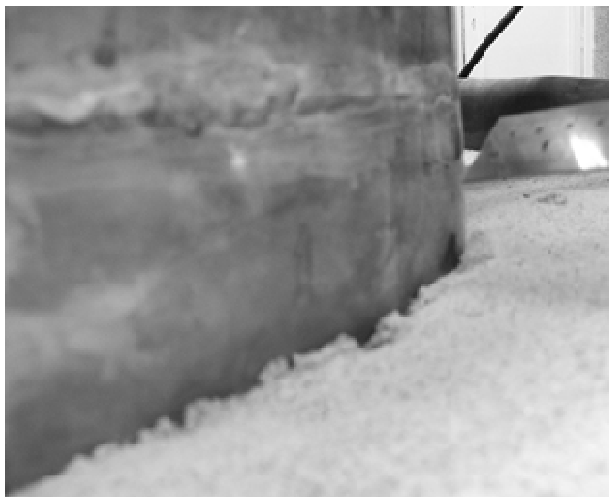
Figure 4. Slipping of the tank in the second experiment on the second tank.
