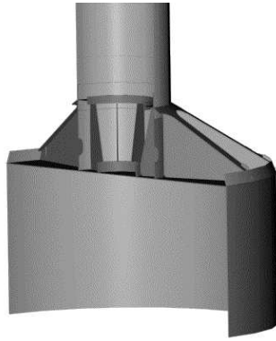
Figure 1. Sectional view of bucket foundation
