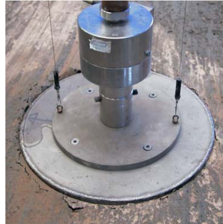
Figure 5. Bucket foundation before and after installation
