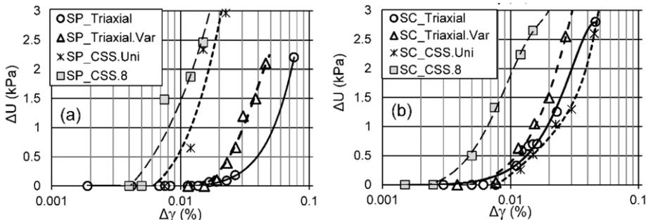
**Figure 4.** Cyclic shear strain amplitude versus Excess pore water pressure for a conventional triaxial test, triaxial tests an irregular load (Var), unidirectional CSS test (CSS.Uni), and CSS test with an eight loading pattern (CSS.8).
