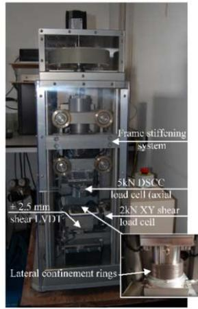
**Figure 1.** University of Dundee Bidirectional cyclic simple shear apparatus.
