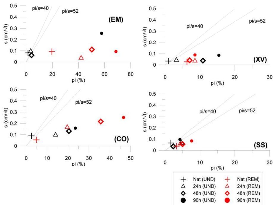
Figure 4. Erodibility test data for undisturbed (UND) and remolded (REM) soil specimens.
