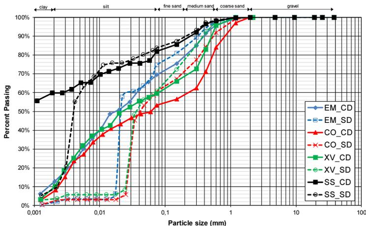
Figure 2. Grain-size distribution curves of the studied soils.
