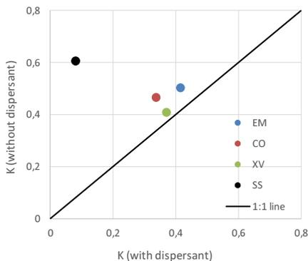
Figure 3. Effects of the use of the dispersant solution for the particle size determination in the calculation of K parameter.
