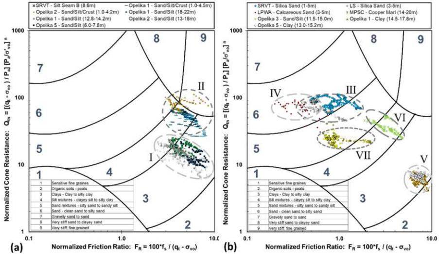
Figure 5. Robertson (1990) soil classification chart with data from: (a) intermediate soils, and (b) silica sands, cemented sand, intermediate soils, and cemented sandy silt.
