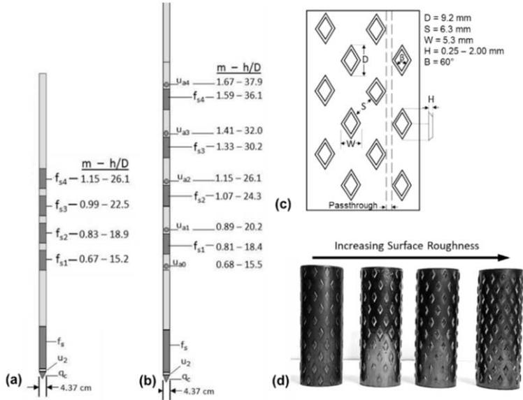
**Figure 1.** Multi-sleeve modules for CPT: (a) MFA and (b) MPFA with distance from CPT tip. (c) Diagram and (d) photograph of textured sleeves.
