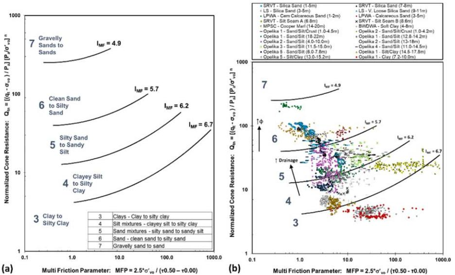
Figure 3. (a) Proposed soil classification chart, and (b) classification of various soils.
