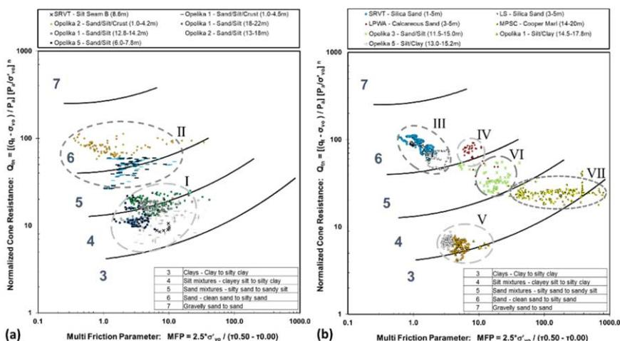
**Figure 4.** Proposed soil classification chart with data from: (a) intermediate soils, and (b) silica sands, cemented sand, intermediate soils, and cemented sandy silt.
