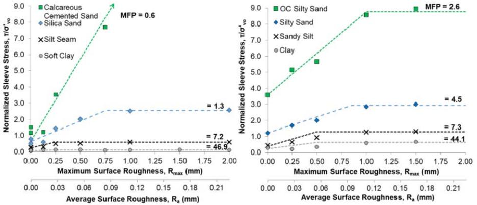
Figure 2. Normalized sleeve stress versus surface roughness from soundings in different geologic strata.
