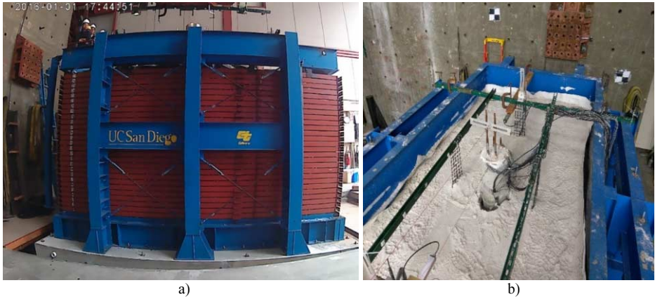
Figure 1. Laminar box on the shake table at UC San Diego a) elevation view b) plan view.
