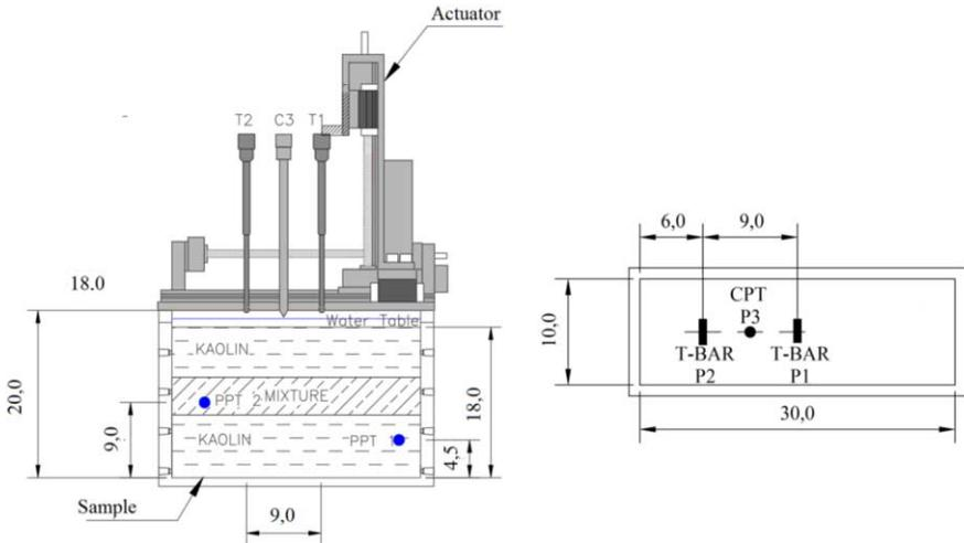
Figure 5. Actuator and location of T-bar and Cone tests.
