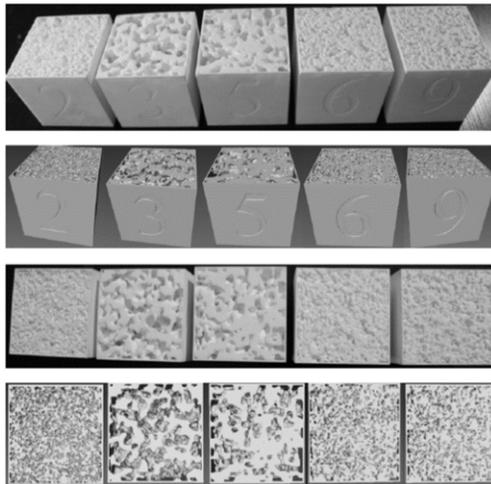
**Figure 4.** 3D prints and computational models for samples 2, 3, 5, 6 and 9 [1].
