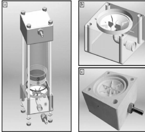
**Figure 2.** Permeameter built by means of 3D printing: (a) basic configuration of the permeameter to be built; (b) computational design of bottom and top of the permeameter and (c) 3D printed result [15].
