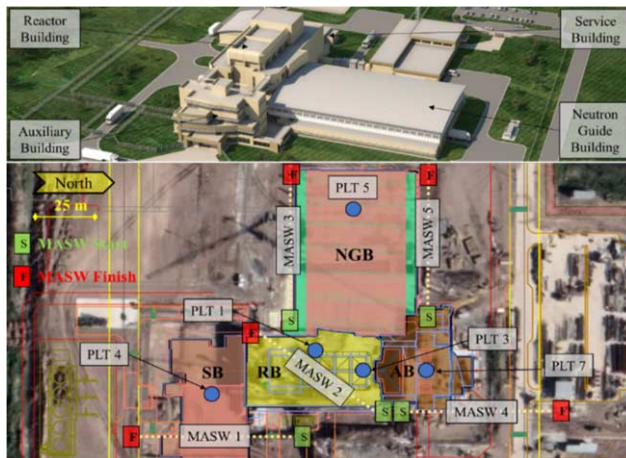
Figure 1. Project layout. Main buildings (up) Location of PLT and MASW testing (down).
