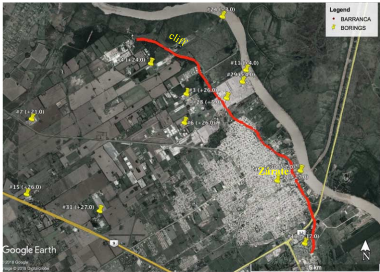
Figure 4. SPT borings on Zárate city.
