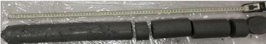
Figure 6. Sample of Postpampeano soil by fixed piston sampler.
