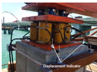
Figure 4. Displacement indicator measurement system
