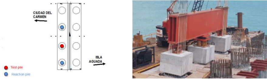
Figure 7. Reaction frame on type 2 abutment.
