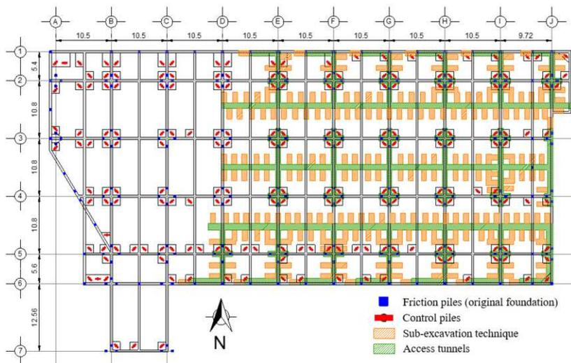
Figure 4. Locations of access tunnels and sub-excitation zones.
