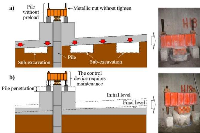
**Figure 6.** Sub-excavation process: a) initial condition and b) after applying the sub-excavation technique.
