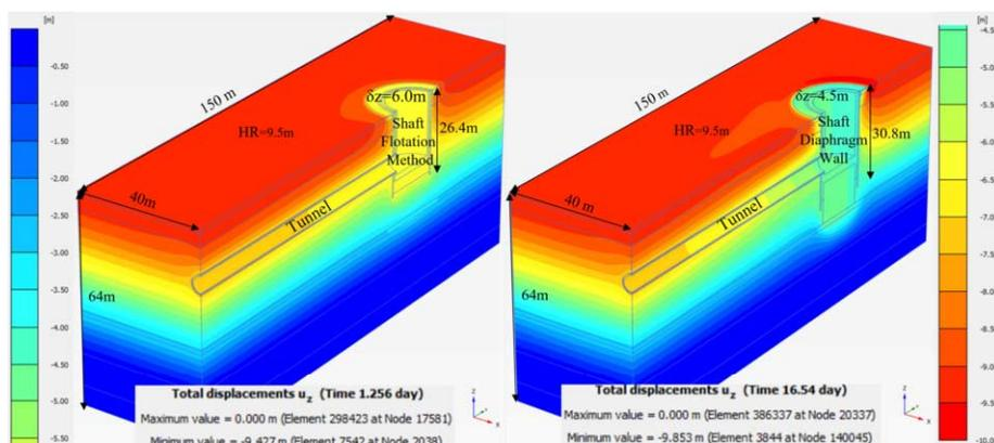
Figure 3. Apparent emersion due to regional subsidence, for the two types of shafts.
