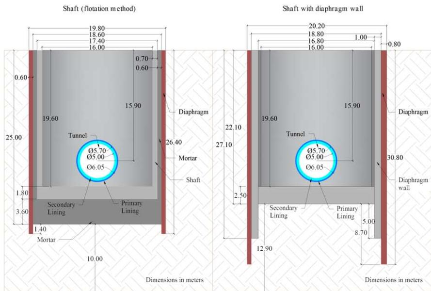
**Figure 1.** Geometric and structural configurations of shafts built with the techniques of flotation and Diaphragm wall.
