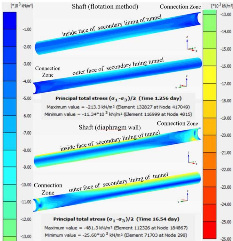
Figure 5. Deviatoric stresses in the tunnel, for the two types of shafts.
