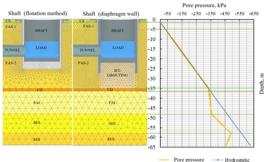
Figure 2. Cases of analysis with the geotechnical model and initial pore pressure.
