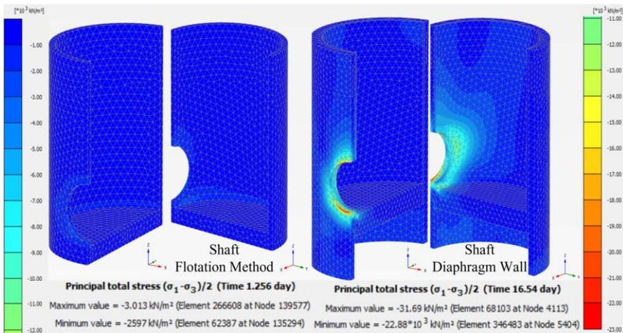
Figure 4. Deviatoric stresses in the tunnel-shaft connection, for both types of shafts.
