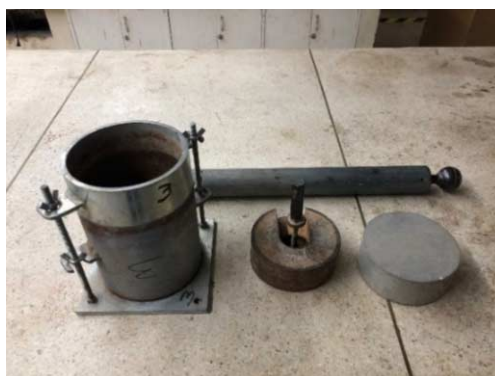
Figure 1. The CBR mold and implements in the CBR Test.
