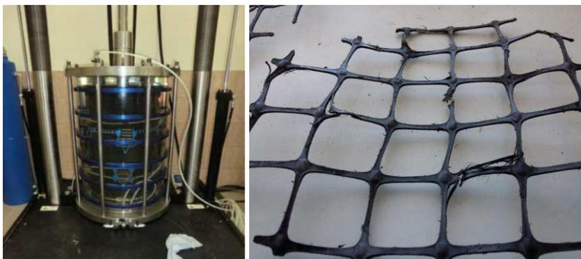
Figure 7. Triaxial shear strength test setup and geogrid after test.
