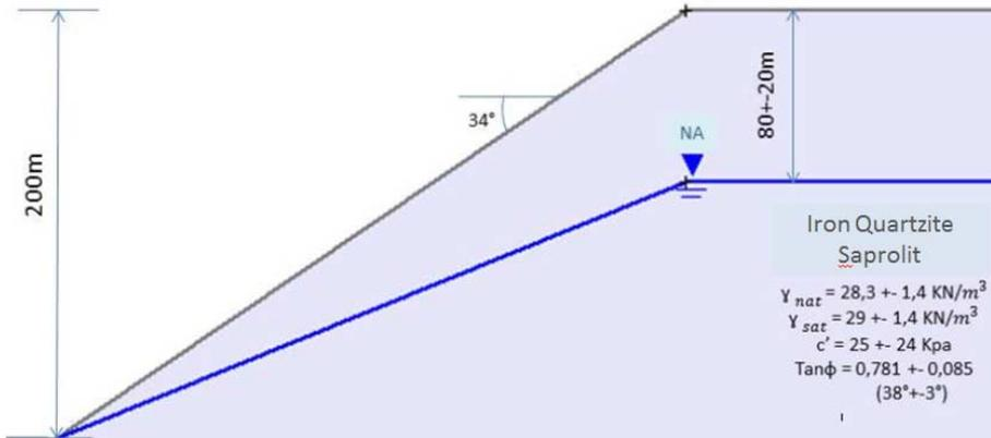
Figure 4. Typical cross section of a slope from the Cauê Mine.
