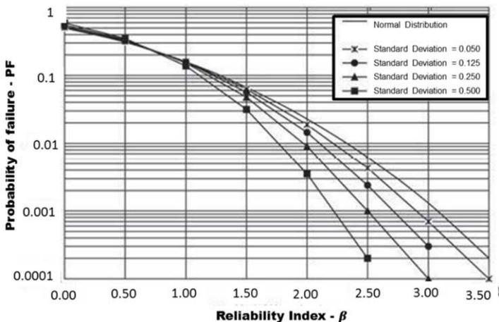
Figure 1. Probability of Failure as a function of the Reliability Index for different assumptions of FS distribution (adapted from [7]).
