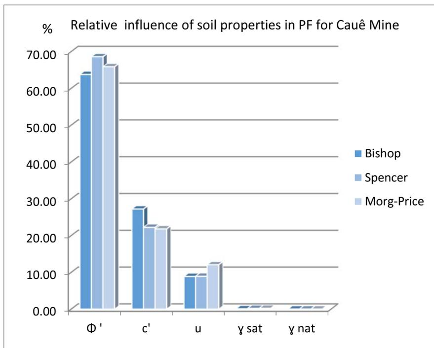
Figure 5. Relative influence of each variable in the Safety of the Cauê Mine slope.
