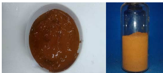
Figure 5. Sample from Jaburu I Dam (left) and the same after drying process and maceration (right).
