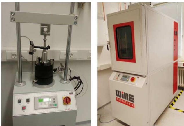
Figure 3. UL-25 oedometer device (left) and UL-60 climate chamber for storing samples (right).
