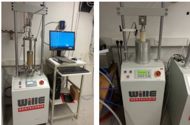
Figure 2. UL-60 (left) and UL-25 (right) uni-axial testing devices for large and small sample sizes, respectively.
