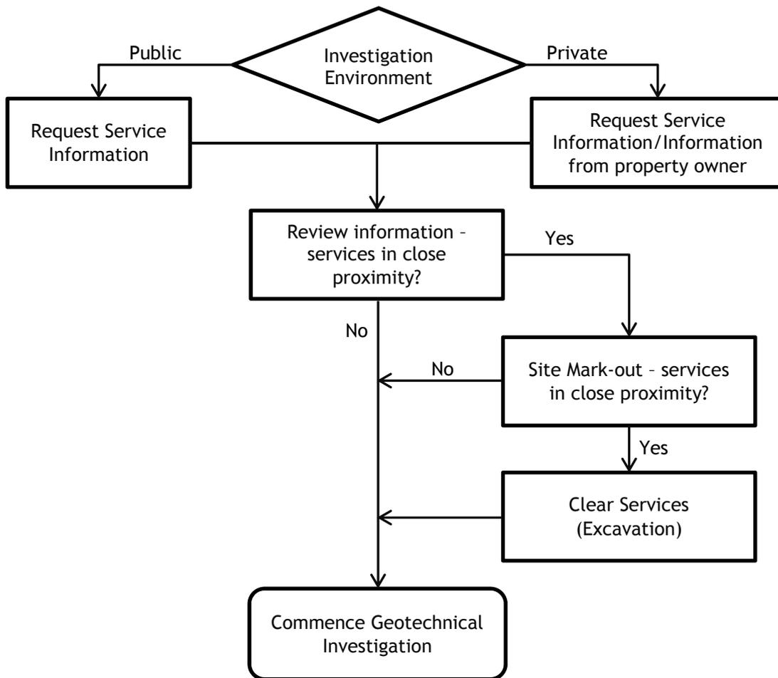
Figure 1. Summary protocol for services avoidance in advance of exploration work
