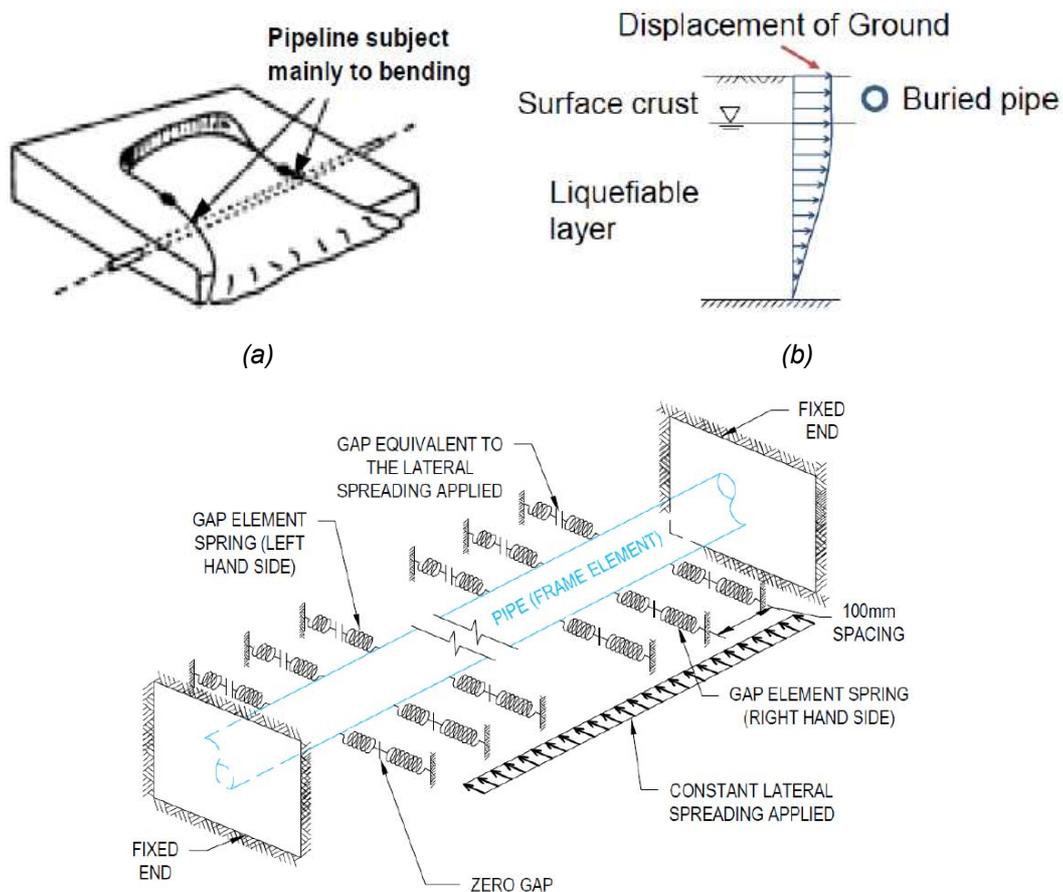
Figure 3. (a) Schematic diagram of pipeline subjected to transverse lateral spreading; (b) location of pipeline in laterally-spreading liquefied ground; and (c) numerical model for SAP2000 analysis.
