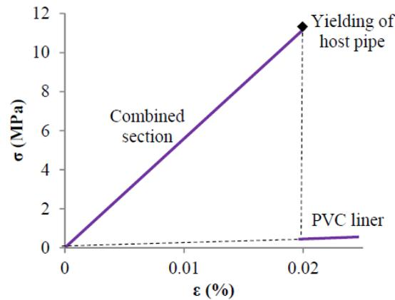
Figure 7. Simplified stress-strain relation for the vitrified clay pipe with AM-liner.
