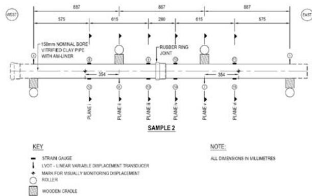
Figure 2. (a) Test set-up for the 4-point load test (Sample 1); and (b) location of sensors (Sample 2).
