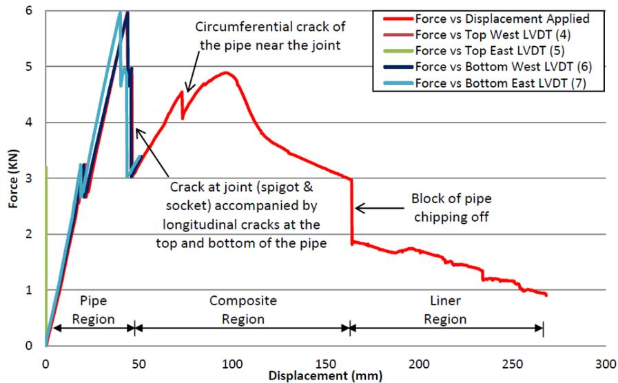
Figure 5. Force-displacement curve for the AM-lined pipe subjected to 4-point loading.
