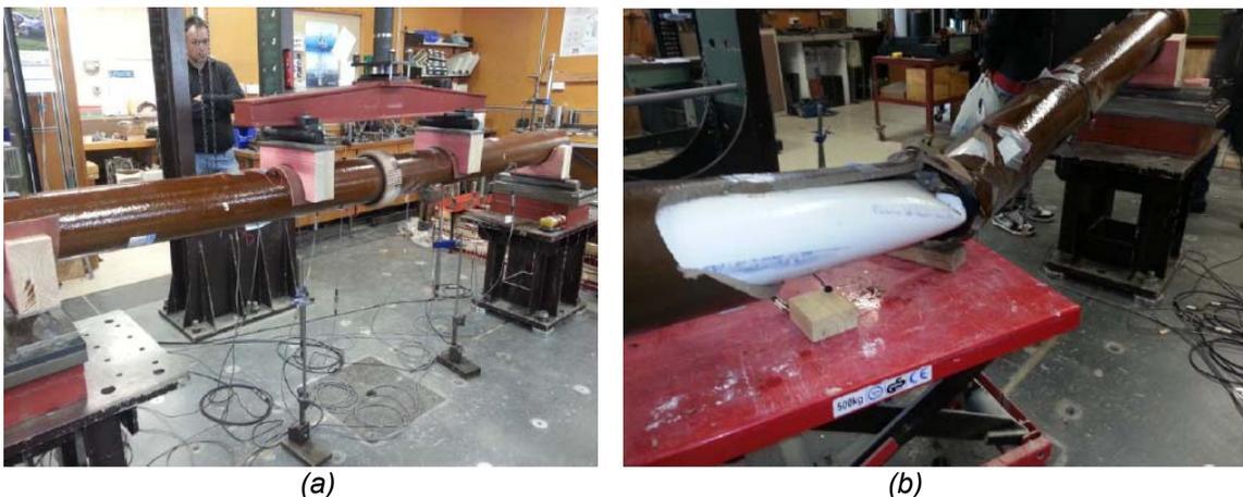
Figure 6. Photos of load test for AM-lined sewer pipe: (a) before the test; and (b) after the test
