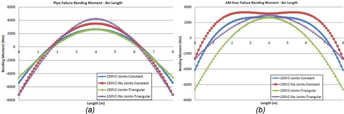
Figure 8. Bending moment distribution of the 8m long pipe: (a) at failure for the unlined pipe; and (b) at failure for the lined pipe.
