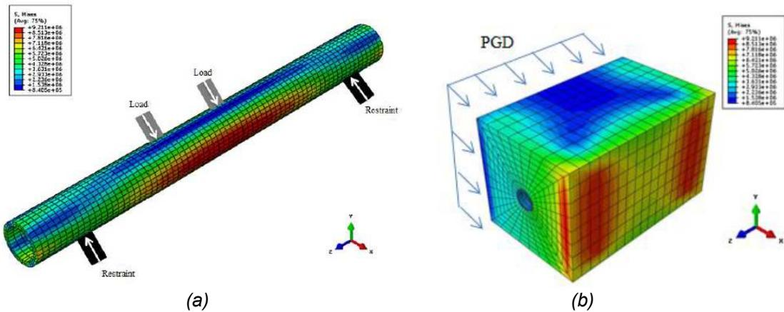
Figure 4. Model in ABAQUS: (a) computer model of the 4-point load test; and (b) model for the pipe subjected to lateral spreading.
