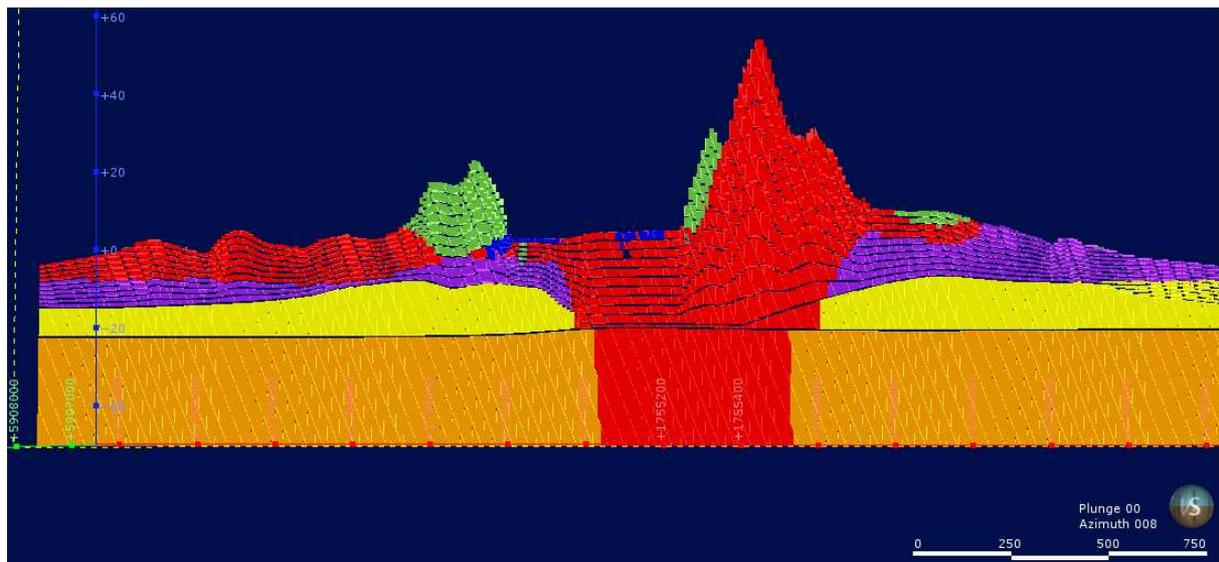
Figure 5. Groundwater flow model layer zonation in Leapfrog (same location as Figure 4). Colours represent different lithological units.
