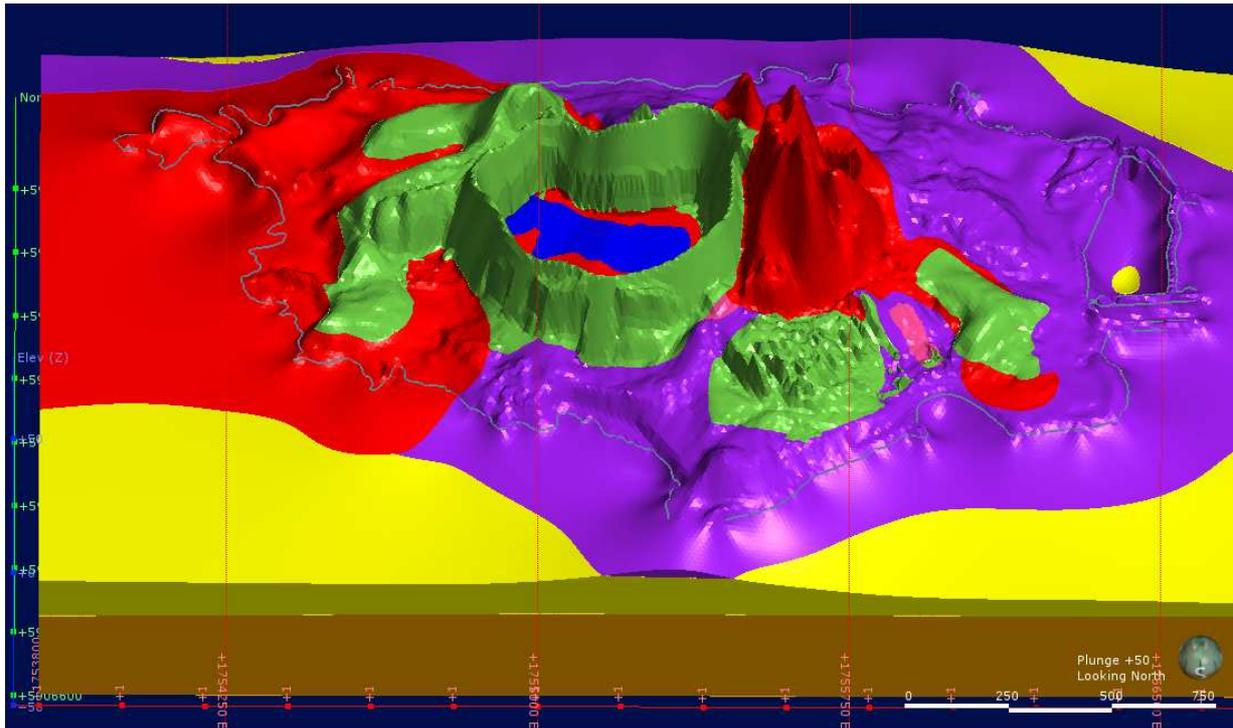
Figure 3. Leapfrog viewer output showing a 3D geological model of the site and biosolids containment facility embankment - oblique view looking north. Colours represent different lithological units. The outline of the island can be seen as a thin blue line.
