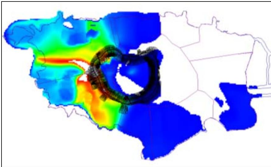
*Figure 6. Groundwater Vistas model output showing concentrations of ammoniacal nitrogen in groundwater under pessimistic case conditions, without the embankment drain. The model was used to determine critical flow paths to optimise the embankment drain location.*
