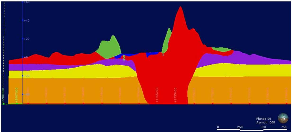
Figure 4. Leapfrog viewer output showing an example 2D cross-section through the geological model of the site and biosolids containment facility embankment. Colours represent different lithological units.
