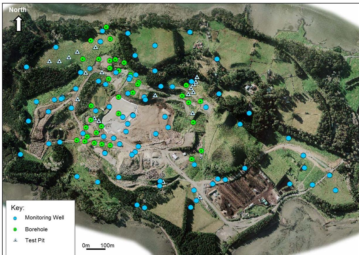
Figure 2. Bore logs from monitoring wells, boreholes and test pits completed since 1997, requiring compilation and interpretation to develop a geological model.
