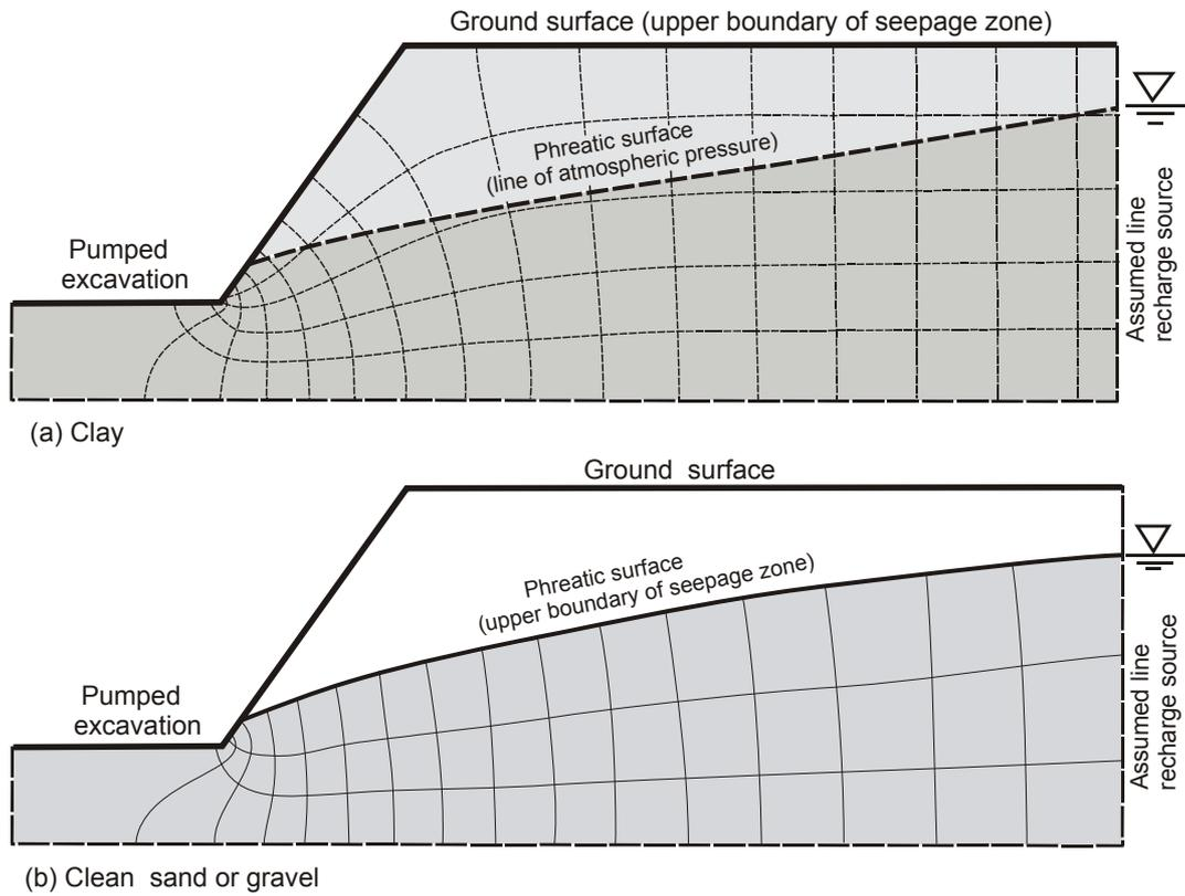
Figure 4. Seepage toward a pumped excavation in clay and in sand or gravel.
