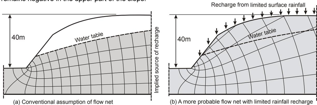
Figure 3. Flow nets compatible with a given water table.
