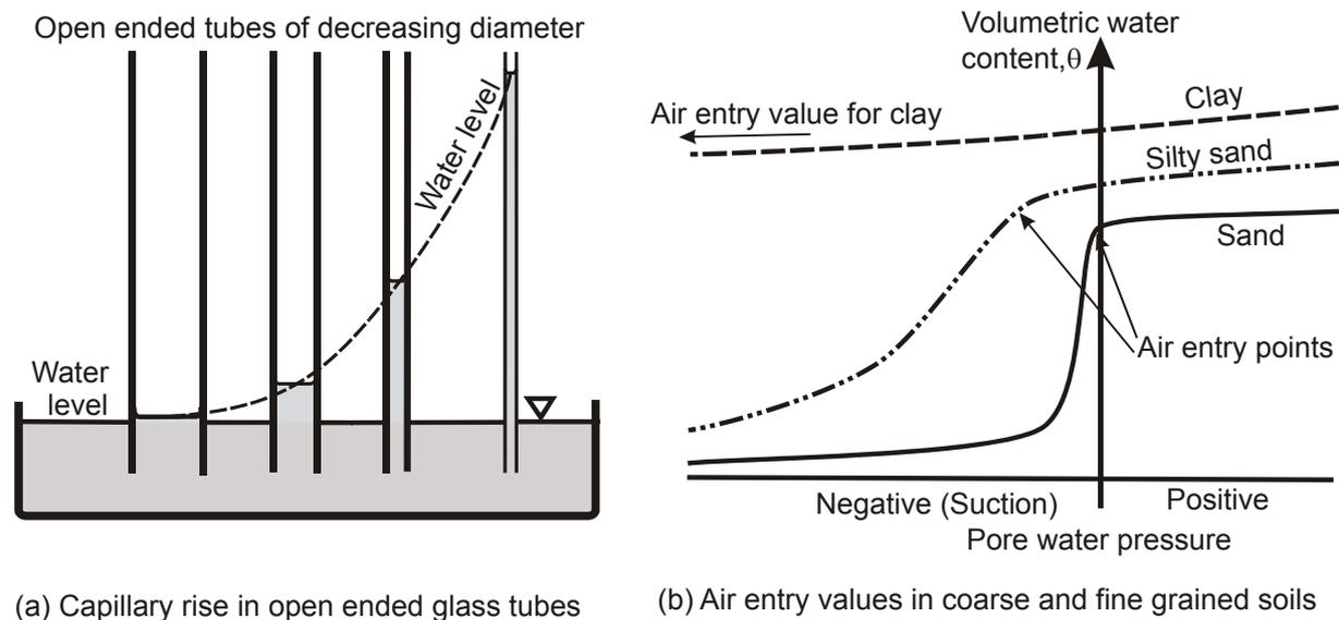
Figure 1. Capillary rise and air entry values in soils.
