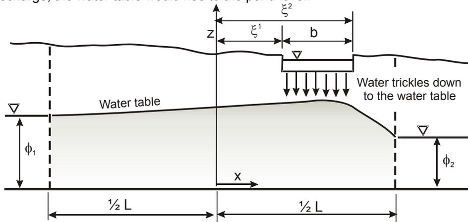
(a) Seepage from a pond, after Strack (1989), for a coarse material
