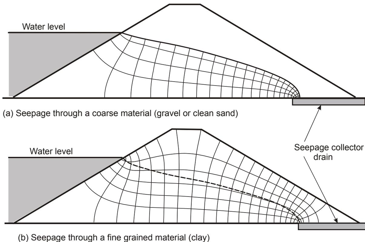
Figure 2. Flow nets in homogeneous embankments built of coarse and fine grained soils.
