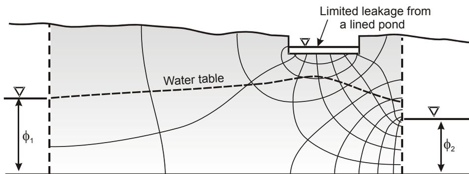
(b) Limited seepage from a lined pond, through clay.
