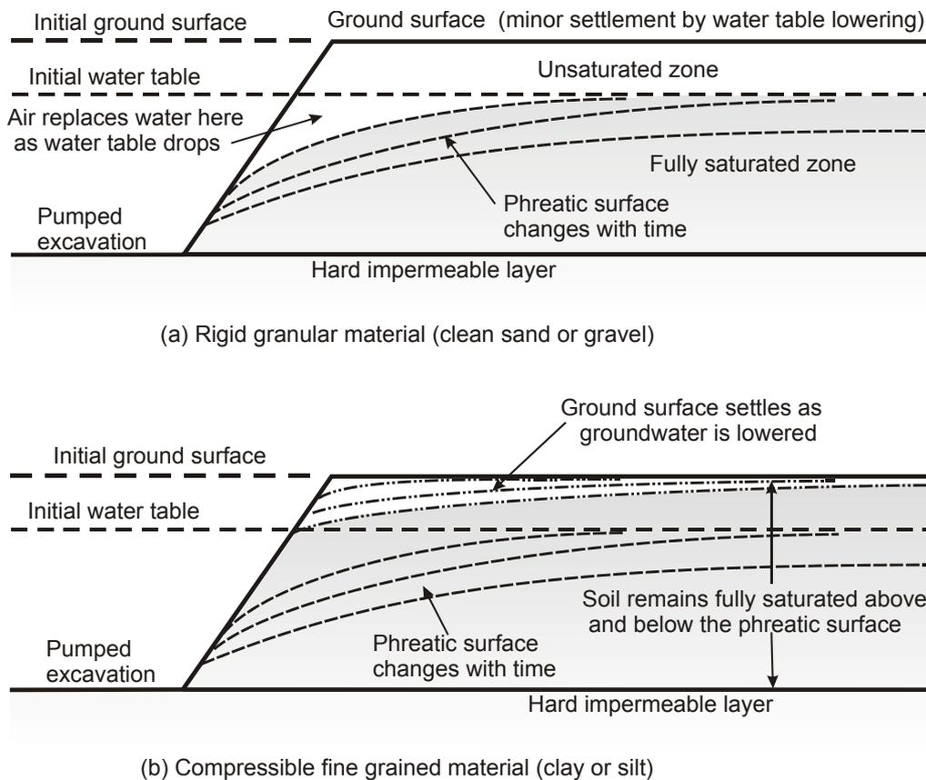
Figure 5. Response of seepage pattern and ground level to dewatering in coarse and fine soil.
