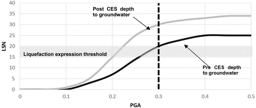
Figure 3b. CPT 36743 LSN vs. PGA for a  $M_w$  7.5 earthquake event for CPT 36743 with a pre and post CES median depth to groundwater of 1.8 to 1.3m
