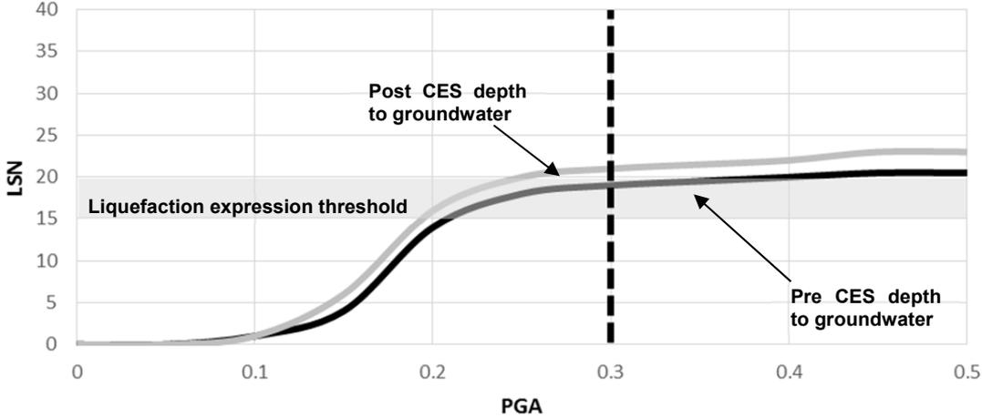
Figure 3a. CPT 5130 LSN vs. PGA for a  $M_w$  7.5 earthquake event for CPT 5130 with a pre and post CES median depth to groundwater of 3.8 to 3.3m
