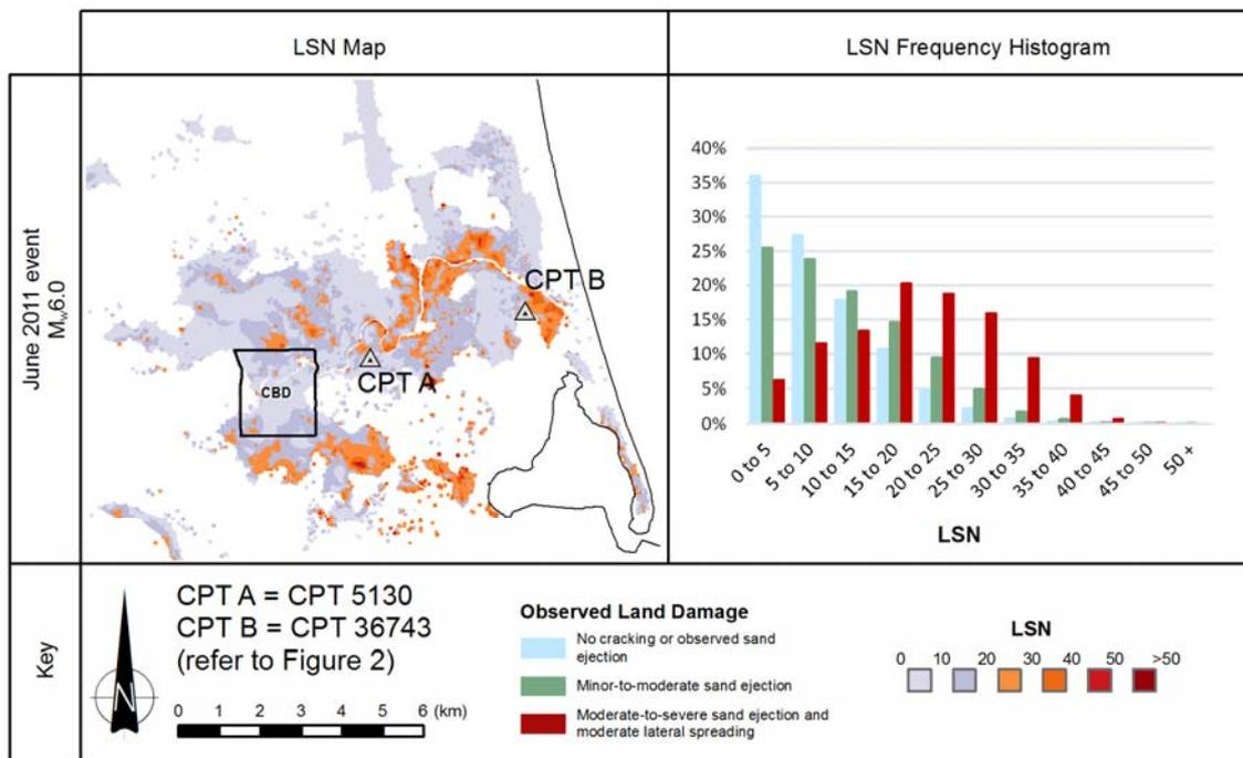
Figure 4. June 2011 earthquake event with adjusted depth to groundwater model. On the left side of the Figure is the LSN map over the top 10m for each CPT using the Boulanger and Idriss (2014) simplified liquefaction evaluation method. On the right side of the Figure is the LSN frequency histogram for the observations of no liquefaction, minor-to-moderate liquefaction and moderate-to-severe liquefaction manifestation at the ground surface.
