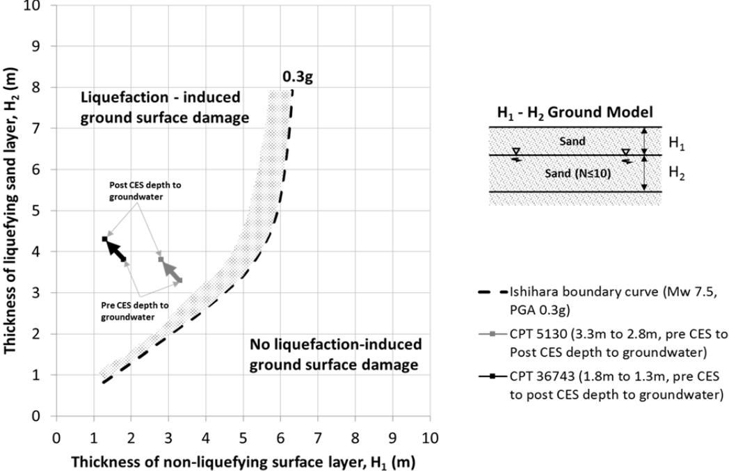
Figure 2. Ishihara (1985) boundary curve for  $M_w$  7.5, PGA 0.3g earthquake event (note the reference numbers used to identify the CPT correspond to the CGD reference numbers).
