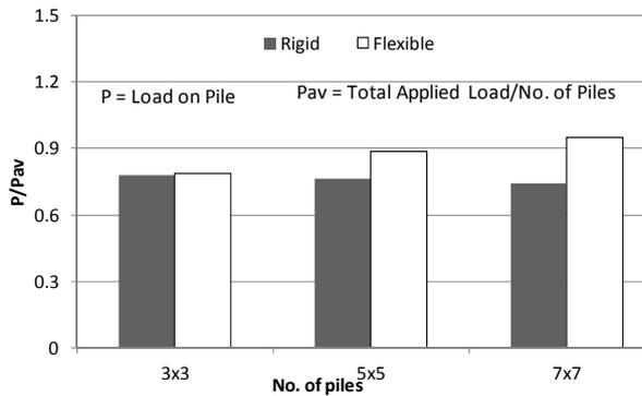
Figure 2. Axial load distribution in centre pile
