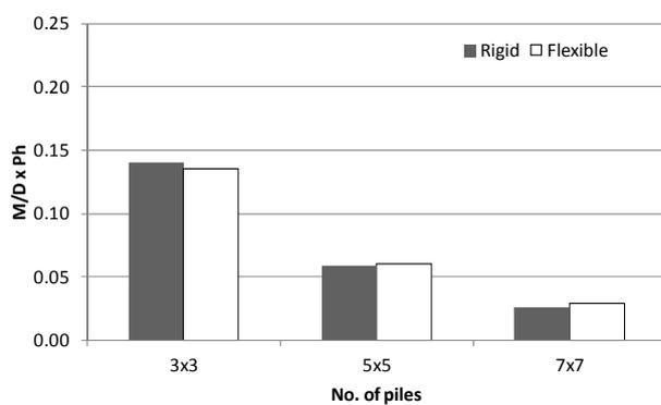
Figure 5. Bending moment distribution in centre pile
