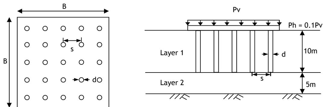
Figure 1. Typical Foundation Layout Embedded in Two Layered Soil Model
