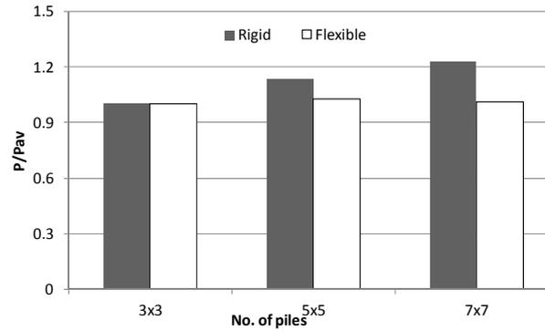
Figure 3. Axial load distribution in corner pile
