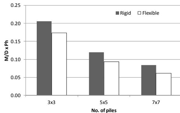
Figure 6. Bending moment distribution in corner pile
