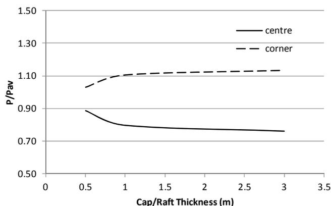
Figure 4. Axial load distribution in piles with different raft thickness for Case 2 – 5x5 pile group
