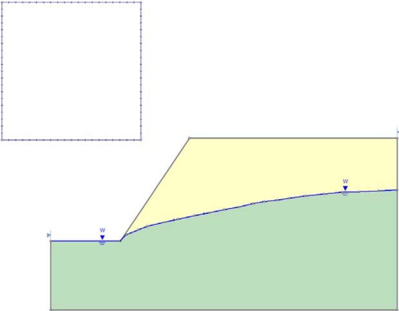
Figure 1. Physical slope geometry and groundwater level
