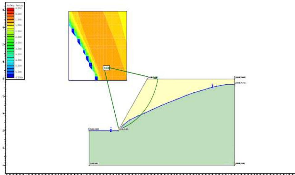
Figure 4. Example of the slope,  $\beta = 56^\circ$  with water level of 4X slope height behind toe of slope
