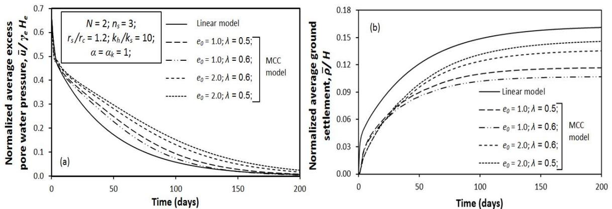
Figure 12. Comparison of linear and MCC models for time-variation of: (a) average excess pore water pressure. (b) average ground settlement.
