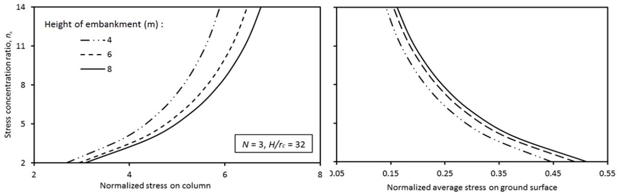
Figure 6. Vertical stresses on column and soil (modified after Indraratna et al. 2013)
