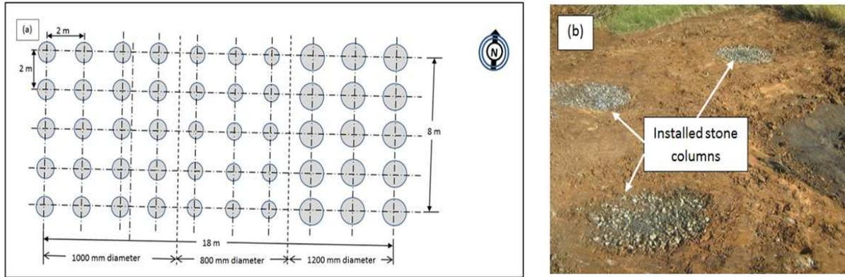
Figure 5. The installed test columns: (a) Plan. (b) Photographic view.
