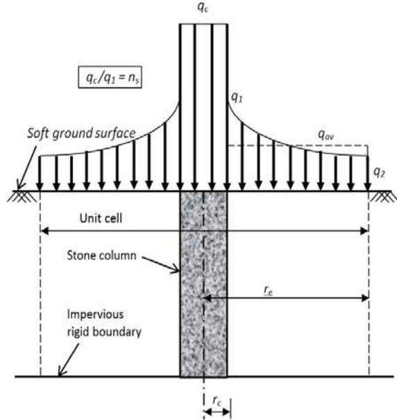
Figure 3. Vertical stress distribution on unit cell surface
