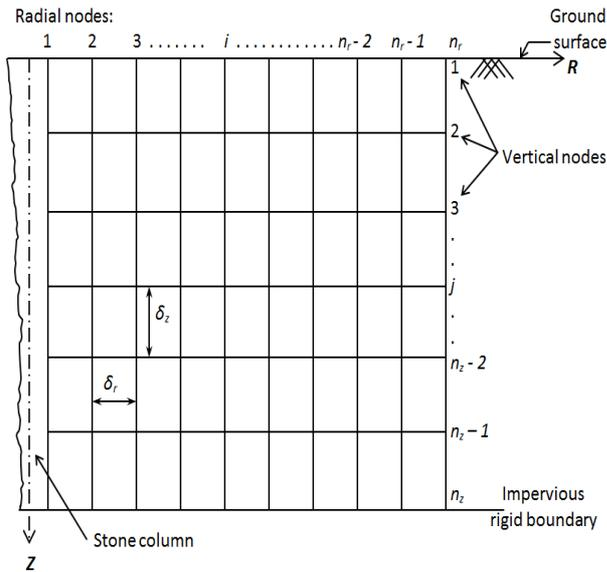
Figure 2. Finite Difference discretization
