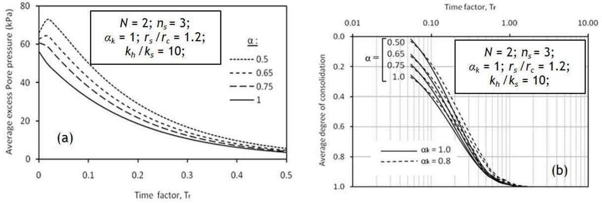
Figure 7. Time variation of: (a) excess pore water pressure. (b) degree of consolidation.
