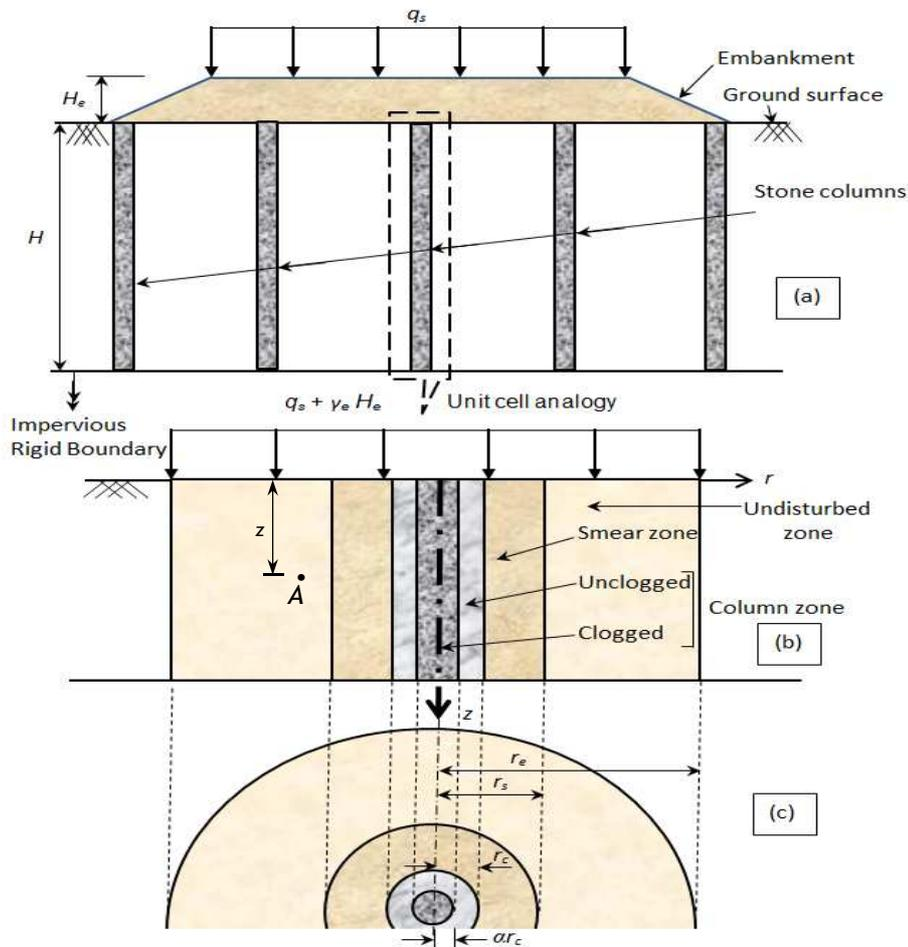
Figure 1. Soft clay reinforcement: (a) Embankment resting on stone column installed ground. (b) Unit cell analogy. (c) Cross section of unit cell.
