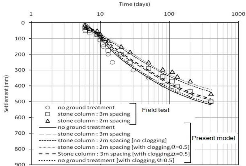
Figure 4. Comparison with field data (modified after Indraratna et al. 2013)
