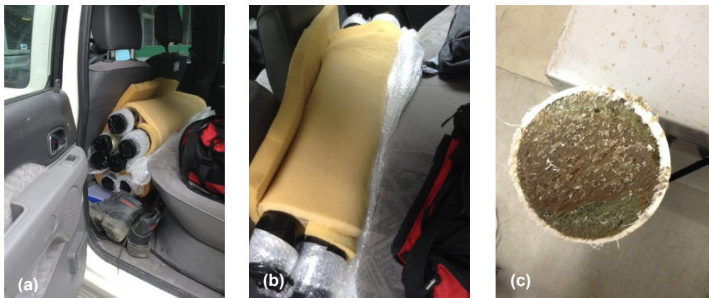
Figure 4. (a&b) Transportation of sample tubes from the site to the laboratory; (c) one end of the sample sliced through to check that transportation had not caused disturbance.
