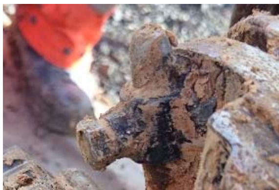
Figure 2. Adjustable spike on the drill head
