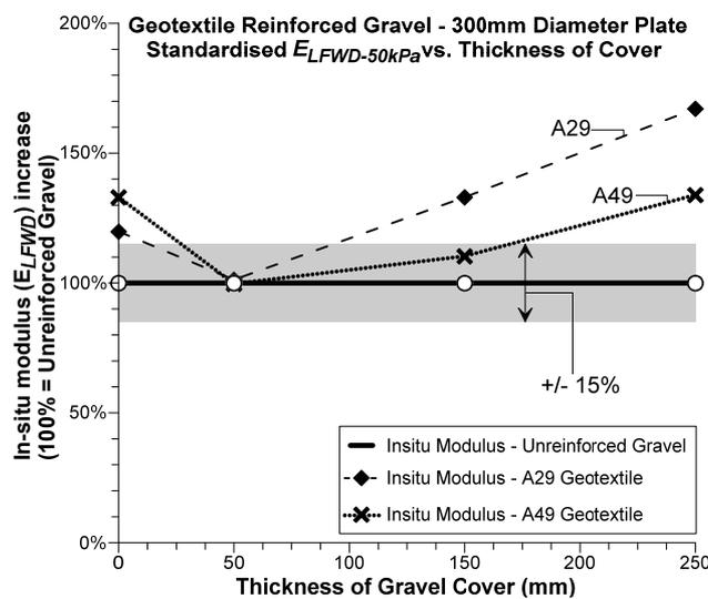
Figure 6. Increase (%) of standardised in-situ modulus ( $E_{LFWD-50\text{kPa}}$ ) based on gravel cover thickness for 50kPa tests completed upon geotextile reinforced and unreinforced 5mm gravel (loosely placed).
