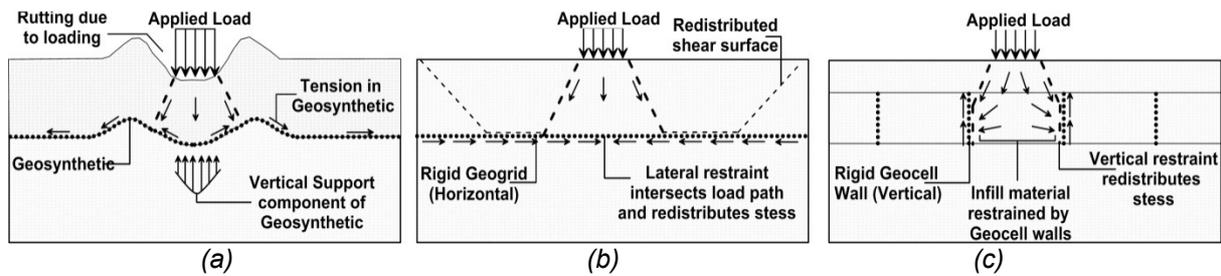
Figure 2. Various boundary conditions through which geo-reinforcement materials provide restraining forces to the surrounding materials; (a) Geotextile tensioned membrane effect; (b) Geogrid confinement via horizontal constraint; and (c) Geocell (vertical) walls preventing material movement.
