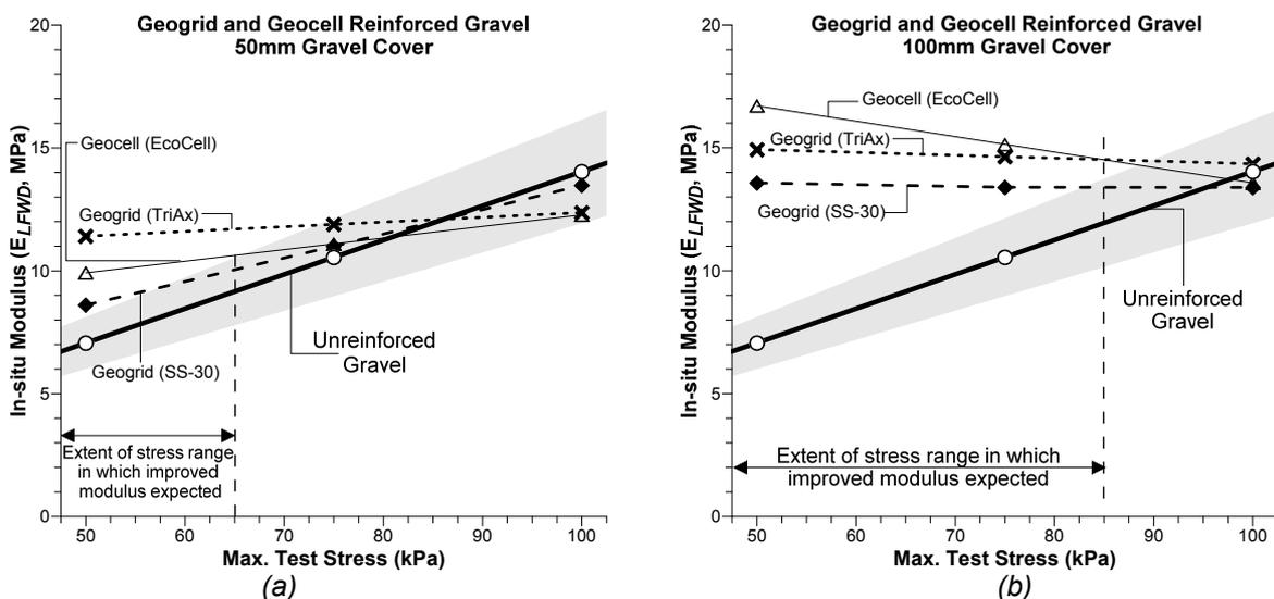
Figure 8.  $E_{LFWD}$  values based on type of geogrid and geocell inclusion, compared to unreinforced material; (a) For 50mm gravel cover; and (b) For 100mm gravel cover (tested using 300mm dia. plate).
