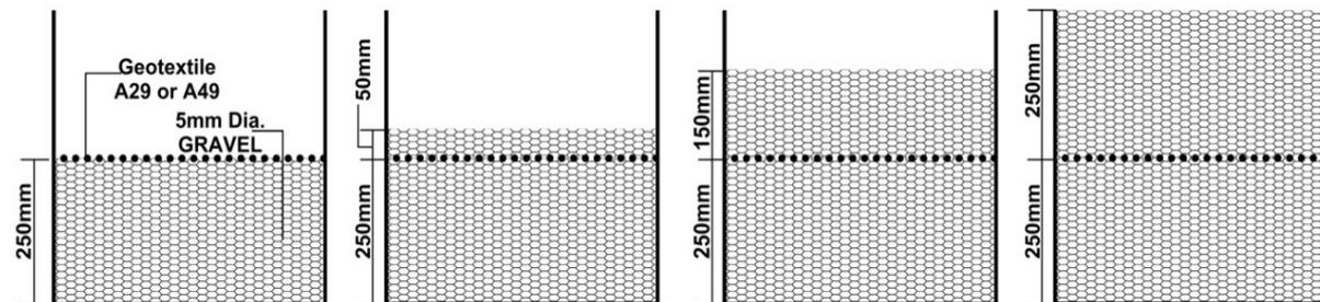
Figure 3. Concept of tested material arrangements (geotextile variation shown)
