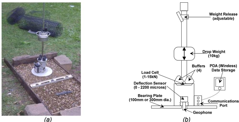
Figure 1. Prima 100 LFWF; (a) during fieldwork and (b) in cross-section (after Fleming et. al., 2007)
