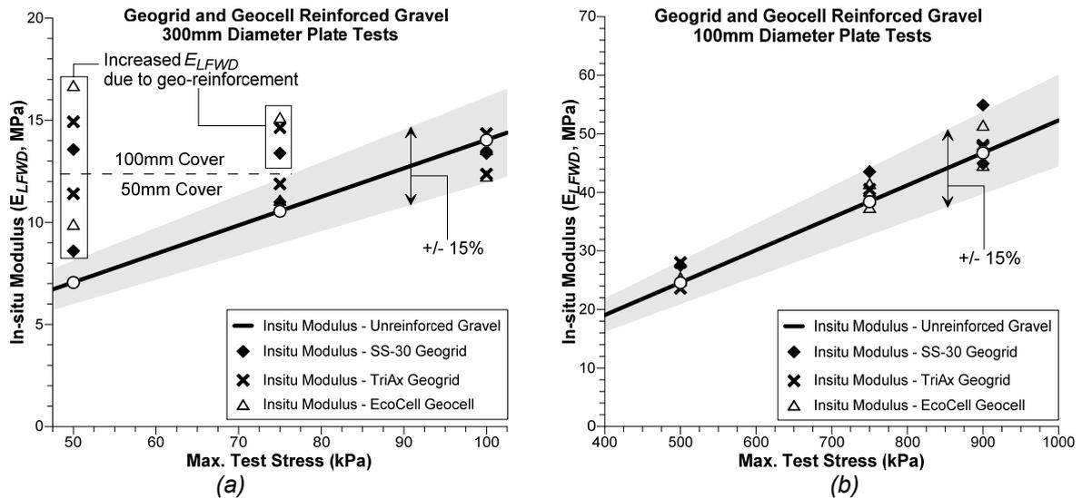
Figure 7.  $E_{LFWD}$  values with geogrid and geocell inclusions, compared to unreinforced material. (a) obtained using a 300mm diameter plate; and (b) obtained using a 100mm diameter plate.
