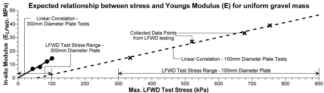
Figure 4. Expected linear relationship between observed  $E_{LFWD}$  values and max. test stress for uniform material within LFWD zone of influence. Note significant change of stress based on utilised plate dia.
