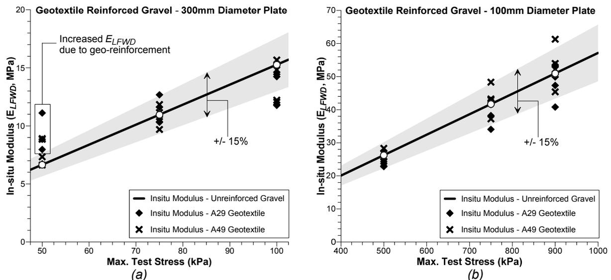
Figure 5.  $E_{LFWD}$  values with geotextile inclusions compared to unreinforced gravel. (a)  $E_{LFWD}$  values obtained using a 300mm diameter plate; (b)  $E_{LFWD}$  values obtained using a 100mm diameter plate.
