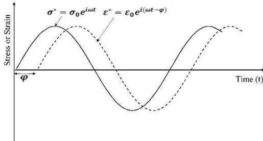
Figure 3. Sinusoidal stress, sinusoidal strain and phase angle
