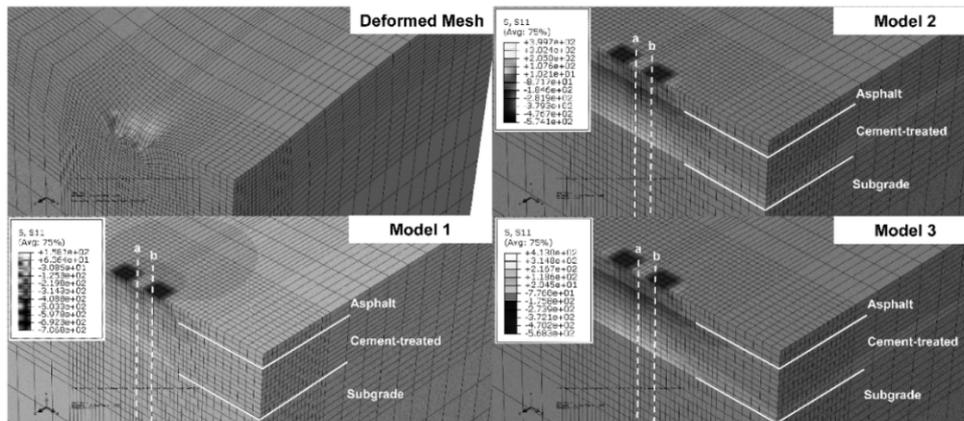
Figure 7. Deformed mesh and horizontal stress distribution induced by the wheel load
