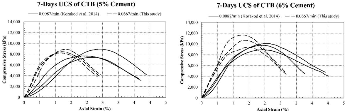
*Figure 1. Strain rate effect to the stress-strain curve of CTB with 5% and 6% cement content*
