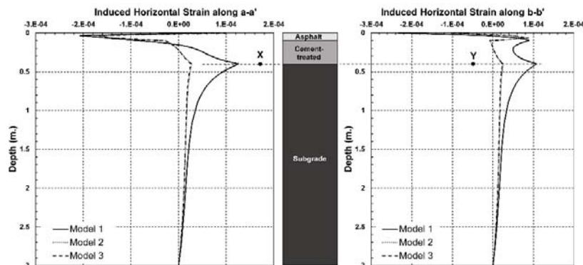
Figure 8. Induced horizontal strain along the section a-a' (Left) and b-b' (Right) of the three models
