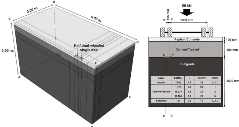
Figure 5. Finite element model, material properties and loading condition
