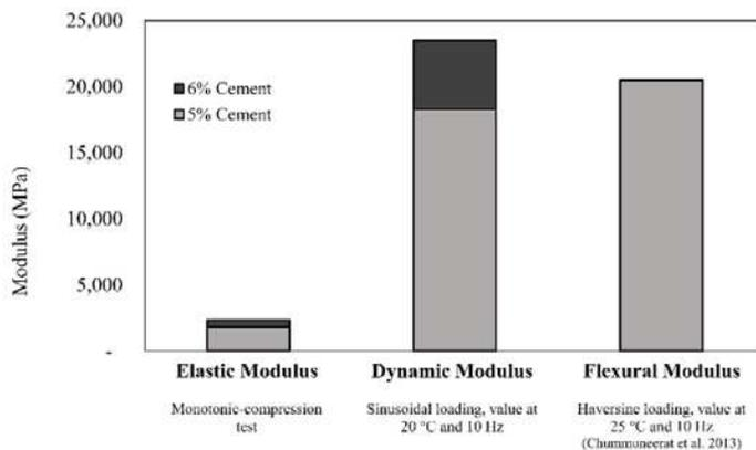
Figure 4. Elastic moduli, dynamic moduli, and initial flexural modulus of cement-stabilised base specimens with 5% cement content and cured at 28 days
