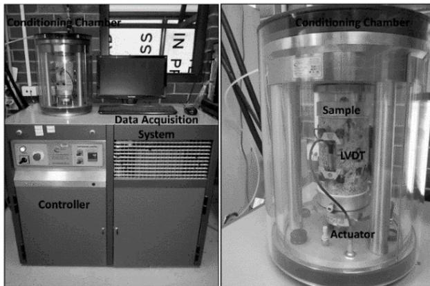
Figure 2. Asphalt Mixture Performance Tester (AMPT)
