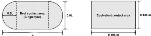
Figure 6. Contact area between single tyre and pavement surface (Left) and equivalent contact area (Right)
