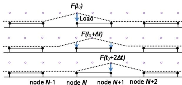
Figure 2. Simulation of moving loads (Araujo, 2011)
