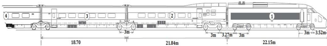
Figure 3. Geometry of Thalys HST (Degrande and Schillemans 2001)
