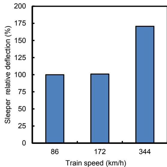
Figure 6. Time history dynamic response of sleeper deflection for different train speed
