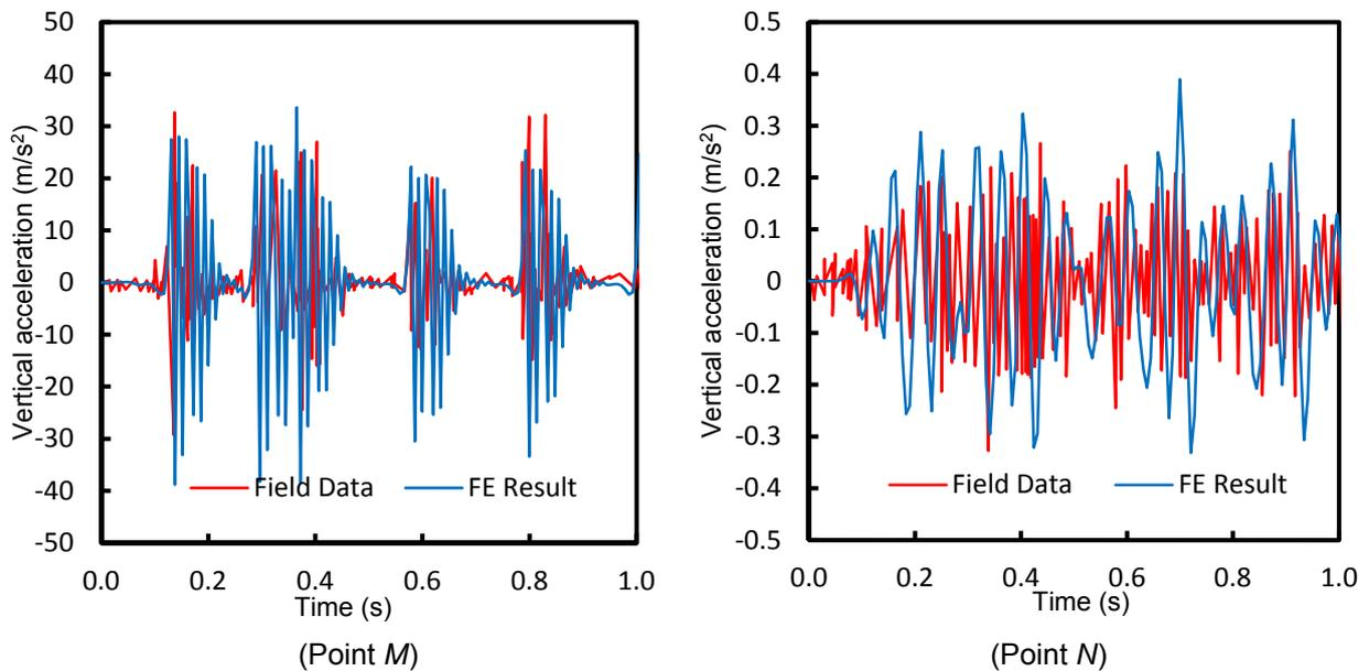
Figure 4. Comparison of FE predicted versus field measured response at observation points  $M$  and  $N$ .
