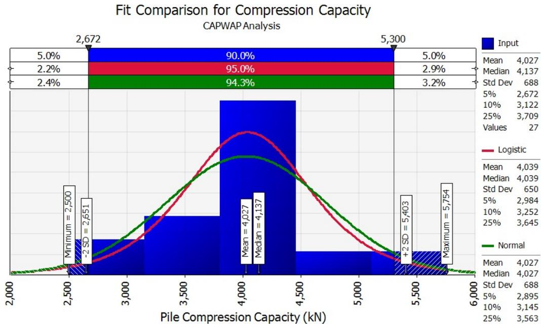
Figure 4. Total Pile Compression Capacity
