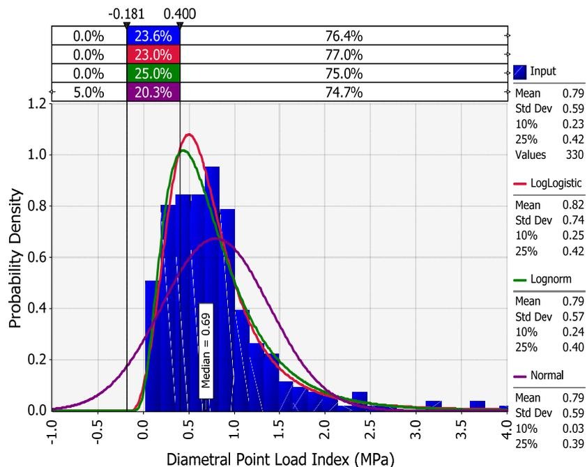
**Figure 1. Comparison of distributions for the diametral  $I_s(50)$  at pier 6**
