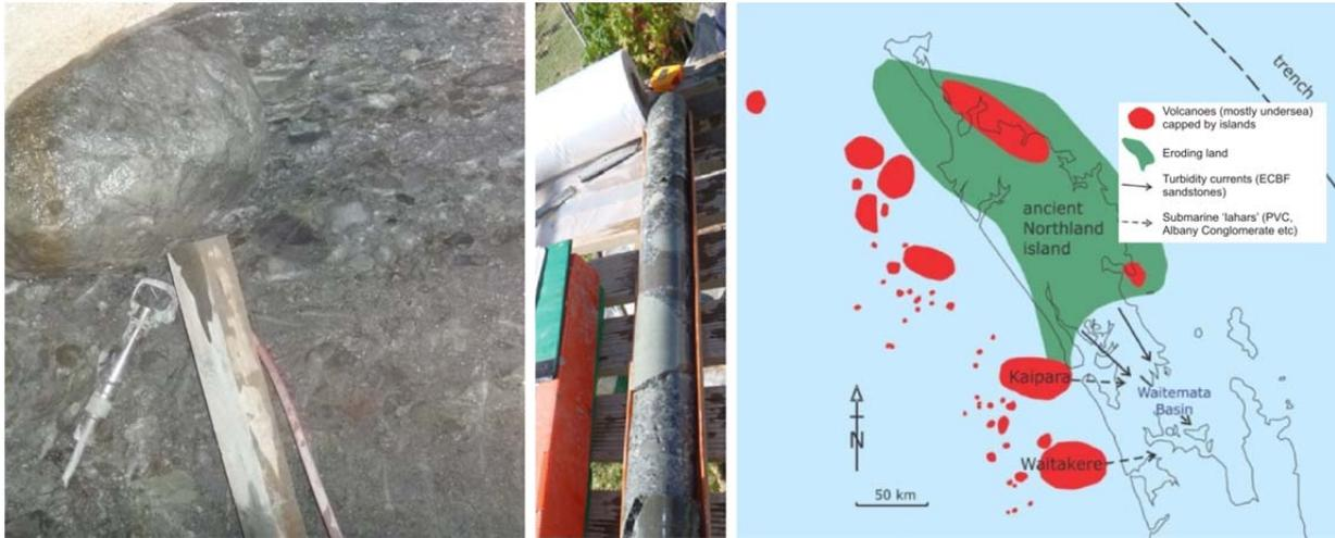
Figure 4. Left and centre: Typical Albany Conglomerate as found in a hand jack tunnel face and core (Roberts et al, 2014). Right: Potential volcanic sources for the Parnell Volcaniclastic Conglomerate shed volcanic detritus into Waitemata basin. Diagram modified from Hayward et al., 2011.
