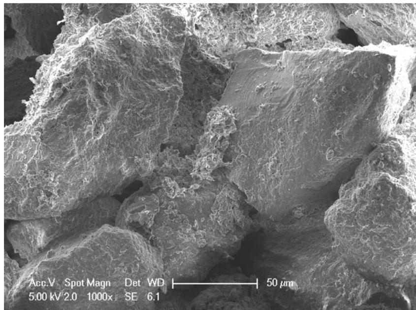
*Figure 2. SEM image of quartz grains recovered from core showing absence of cement and conchoidal impact fracture which could only have happened during deposition; this impact surface is almost clean suggesting that no cementing matrix has existed during the history of this sandstone.*
