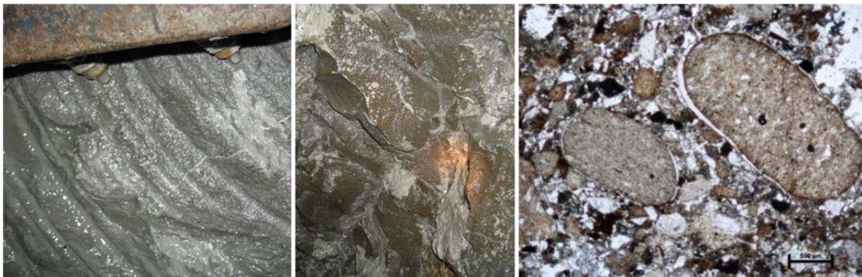
Figure 5. Left and centre: Calcite encountered on Trunk Sewer 30. Right: Microphoto thin-section in plane polarized light. Calcite cemented sandstone clast enclosed in unconsolidated sand. Note white rims of calcite on large rounded lithic (mudstone/siltstone) grains and fragment of volcanic material bottom left.
