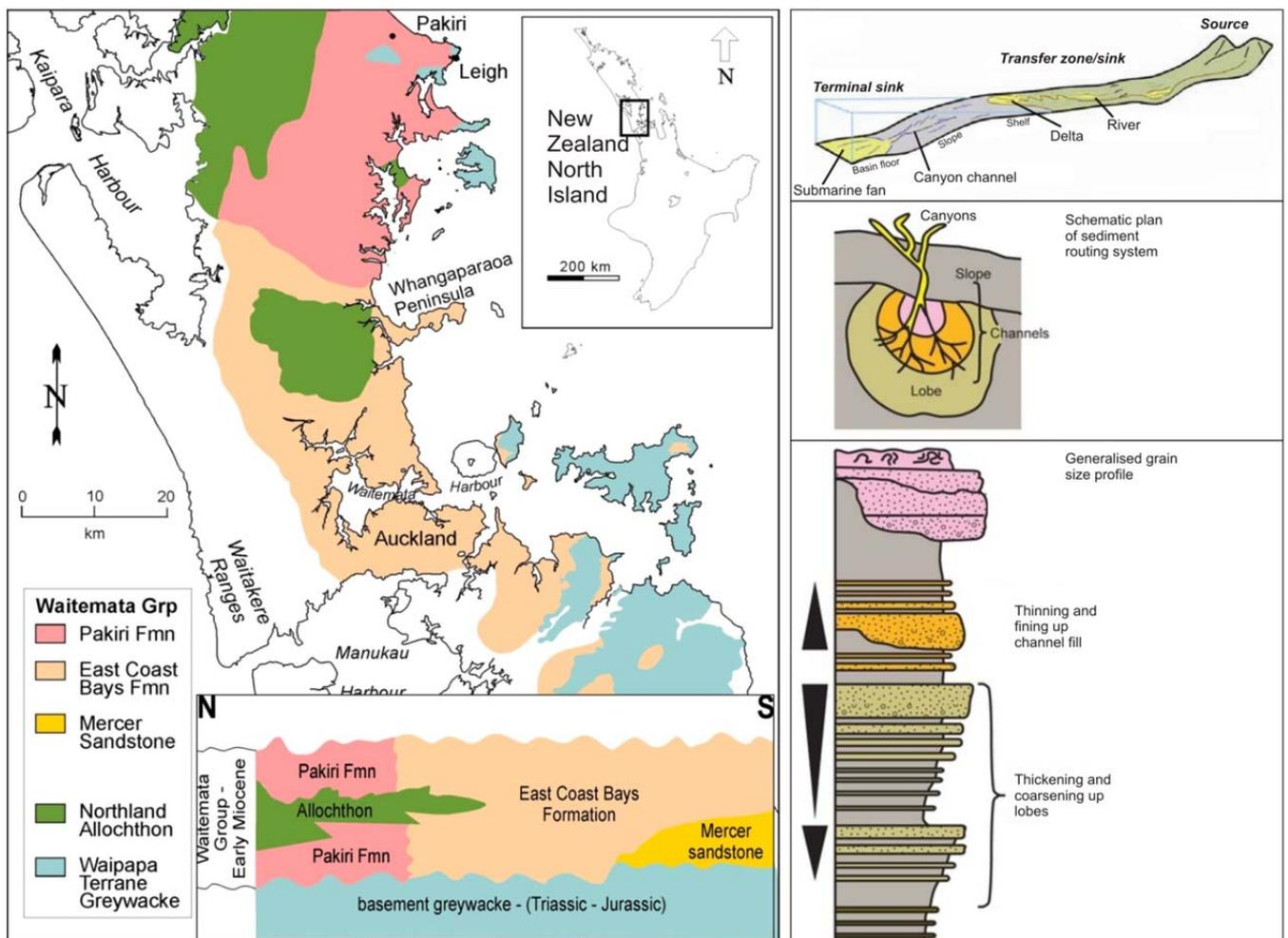
Figure 1. Schematic geological map and section of Auckland, after Edbrooke et al., 2001. Model of submarine fan and turbidite sequence, after. Generalized sediment-routing system (top right) modified from Graham et al. (2011) and Covault (2011). Submarine fan model (middle right) resulting in vertical stacking of sedimentary rocks (bottom right) modified from Mutti (1992)
