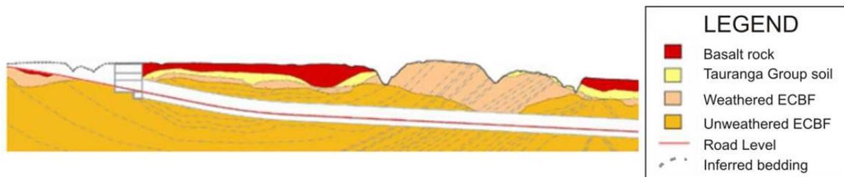
Figure 3. Waterview tunnel long section showing dip and weathering variability, with deeper weathering in zones of high bedding dip. Amended from Kenyon, 2014.
