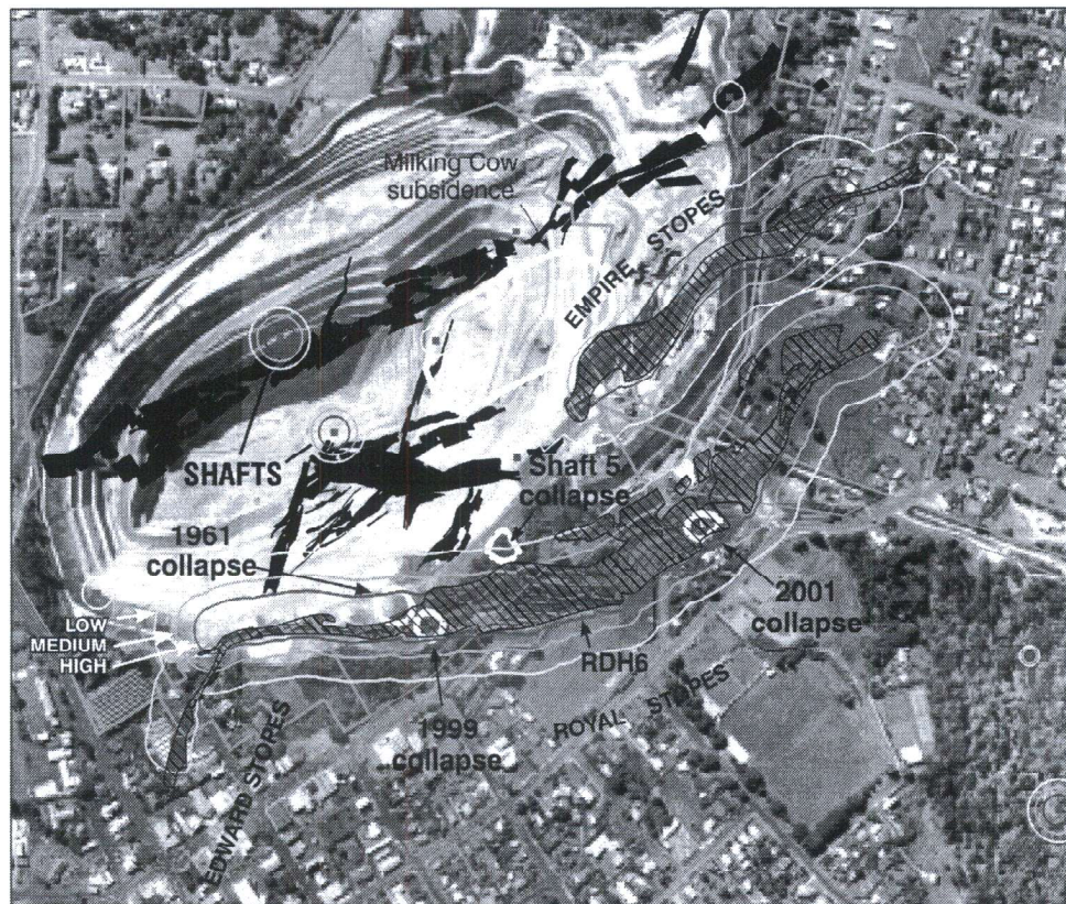
Figure 4. Probabilistic ground subsidence hazard zones overlying mine stopes and shafts
