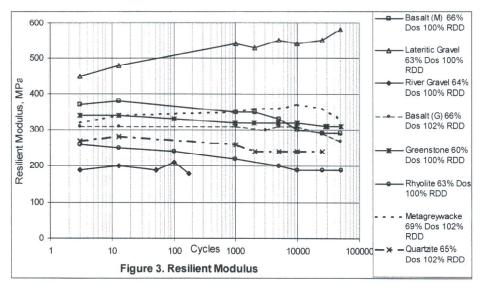
Under cyclic loadings, these materials undergo resilient strains, which are recovered after each cycle, and permanent strains, which accumulate with the number of cycles.
