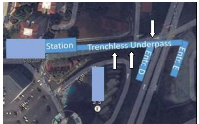
Figure 1 Layout of pedestrian underpass with arrows marking location of knock-out panels for future connections
