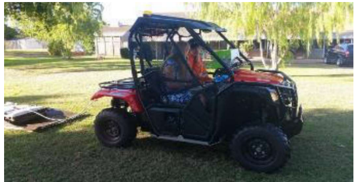
Figure 4 – GPR Field Setup showing towed 80MHz shielded antenna behind the all-terrain vehicle.
