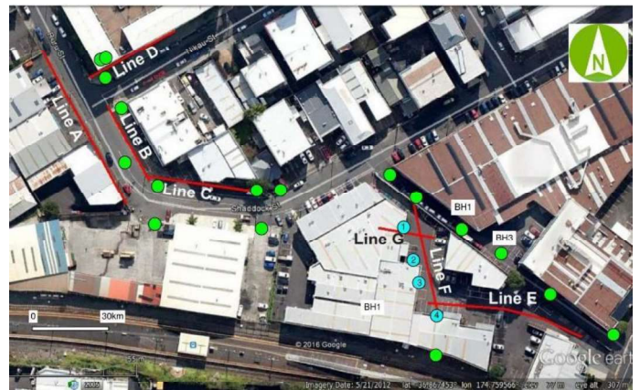
Figure 1. Locations of the ReMi seismic arrays (red) near Mt Eden Train Station. Green dots show boreholes nearest the seismic survey locations at the time of the investigations. The cyan dots show boreholes drilled after the ReMi investigations. Labels refer to the boreholes shown in Figure 2.
