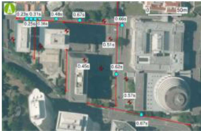
Figure 3. Locations of the ReMi seismic arrays and boreholes (red) at Bowen Campus/Parliament Precinct, Wellington, New Zealand. Site period measurement values across the site are displayed, with estimates from the seismic ReMi data shown as cyan circles. Aerial photograph sourced from LINZ Data Service ( https://data.linz.govt.nz/data/category/aerial ) and licenced under the Creative Commons Attribution 4.0 New Zealand.
