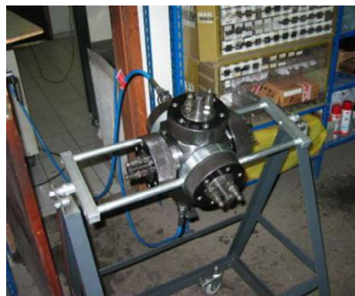
Figure 4. General configuration of Brazilian cell
