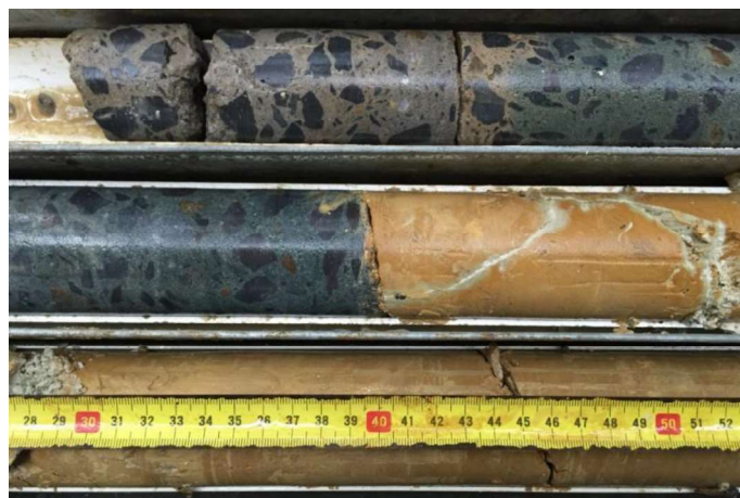
Figure 2. Core photograph showing the contact between the concrete footing and underlying weathered siltstone.
