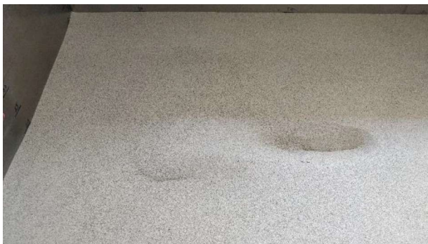
Figure 8. Top surface of test tank after test (shallow anchors)
