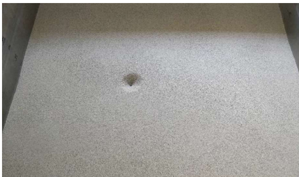
Figure 9. Top surface of test tank after test (deep anchors)
