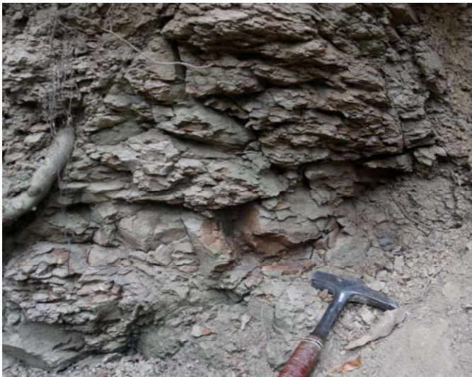
Figure 10. Intensely shattered siltstones at the base of the slide.
