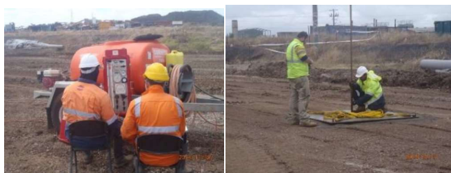
Figure 7. Pressuremeter testing in progress (L), Settlement Plate Setup prior to trial embankment construction (R)
