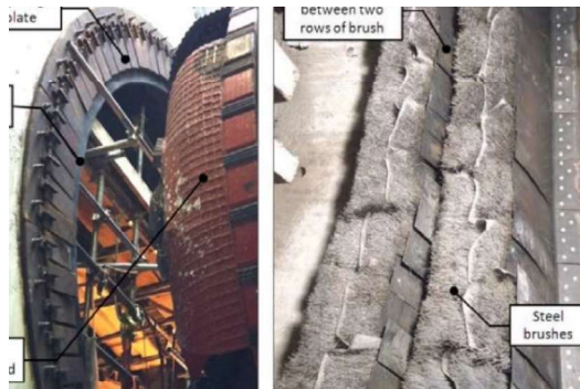
Figure 5. One-way rubber packer (left) and steel wire brushes (right) (after Tsang et al. 2012)
