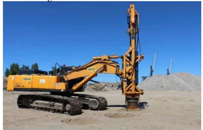
Figure 2. Rapid Impact Compactor.
