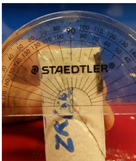
Figure 13. Failure plane for a sample, it can be seen that the angle of the plan with the horizontal is around 67^\circ .
