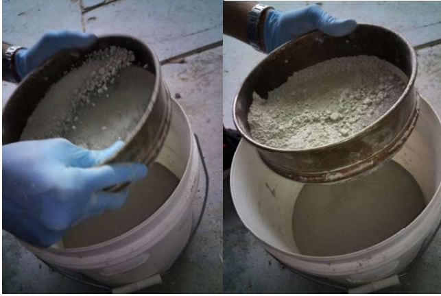
Figure 2. Cement powder before and after the sifting process.
